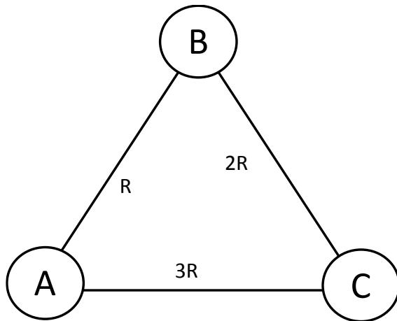
3. Suppose that day-ahead electricity demand was expected to be 9 MWh during some hour, and that the generators submitted supply offers equal to marginal cost. Calculate the quantity cleared by each generator in the day ahead market, flows on the three transmission lines and the day-ahead Locational Marginal Prices at each of the three nodes.
