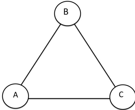
1. Suppose that the marginal costs of the two generators are  $MC(G_A) = \$5/\text{MWh}$  at Node A and  $MC(G_B) = \$15/\text{MWh}$  at Node B. Generator A has a maximum capacity of 15 MW and Generator B has a maximum capacity of 15 MW. Demand at node C is 25 MWh. Flow constraints on the transmission lines are:
